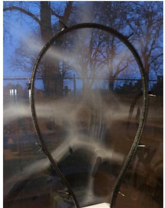
Fig. 2. An AirRevival N7-70/90 unit placed in a preschool window. Note the accumulation of particles on the glass behind the emitter arch.
