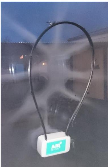
An AirRevival unit attached on a window in a preschool. Note the accumulation of particle, easily wiped off from the glass surface.
